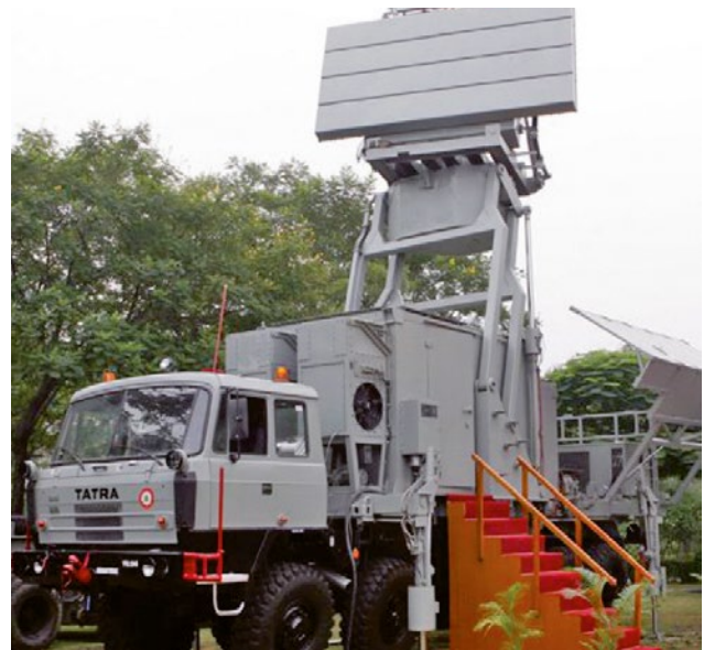
TATRA MOBILE PLATFORM WITH 3-D CAR RADAR
